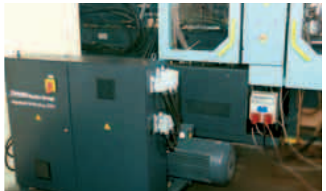
The compact hydraulic unit mounted opposite the operator's side
