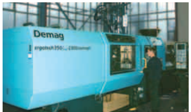
The Demag Multi-plug working in combination with a Concept 350/710-2300
