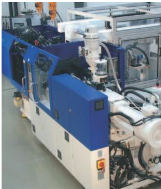
Production cell with EL-EXIS S 150 injection moulding machine, Waldorf-make high-speed parts-removal robot, and Kebo-make IML mould
